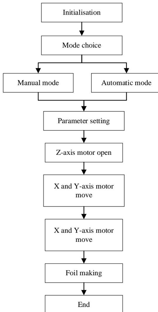
Figure 6: Control operation flow chart.
