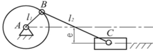
Figure 3: The slider crank mechanism.
