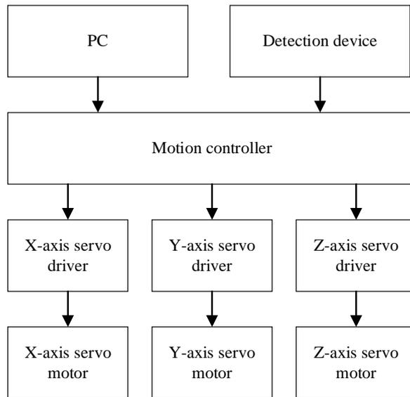
Figure 5: The system control principle.
